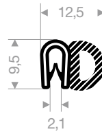
24500135 pvc + sponge rubber clamping range 1-2 mm roll length 50 meter
