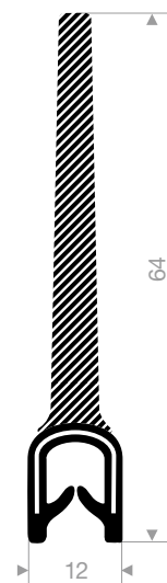
24500865 pvc + sponge rubber clamping range 1-2,5 mm roll length 50 meter
